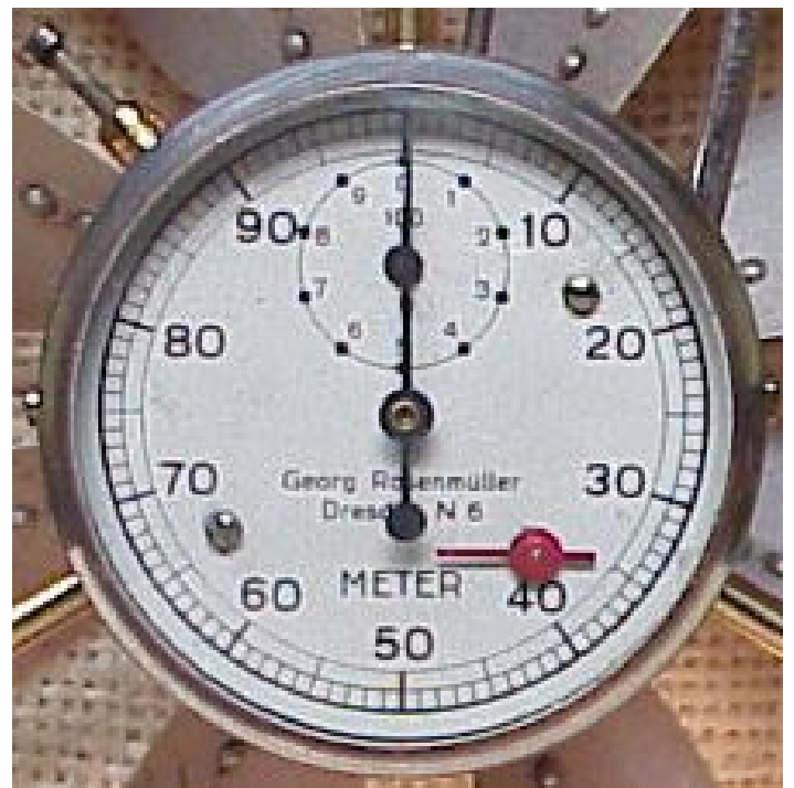
BELOW: Copper and brass Georg Rosemuller 2 dial model with built-in stop watch. Closeup of Rosenmuller anemometer at right.
